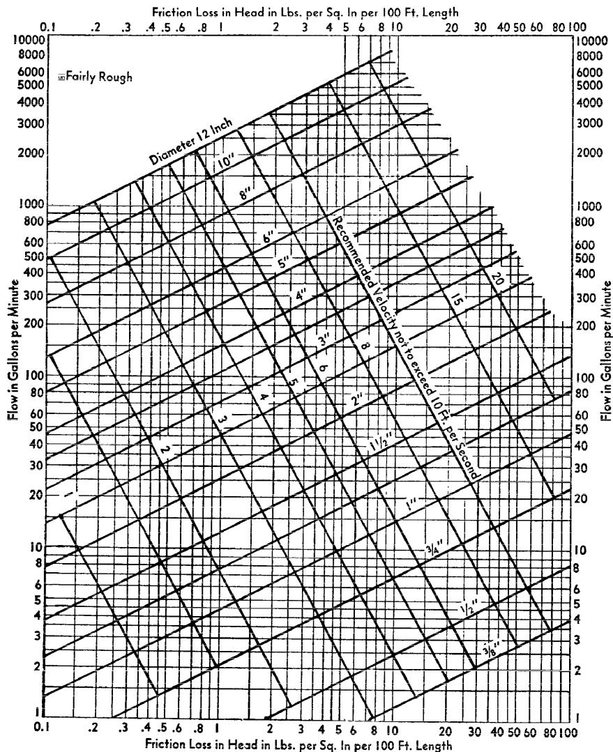
**Subp. 17. Pressure loss of water in pounds per square inch per 100 feet of rough pipe.**
