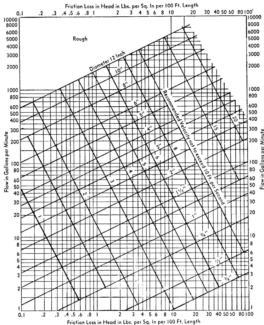
**Subp. 19. Pressure loss of water in pounds per square inch per 100 feet of copper pipe.**
