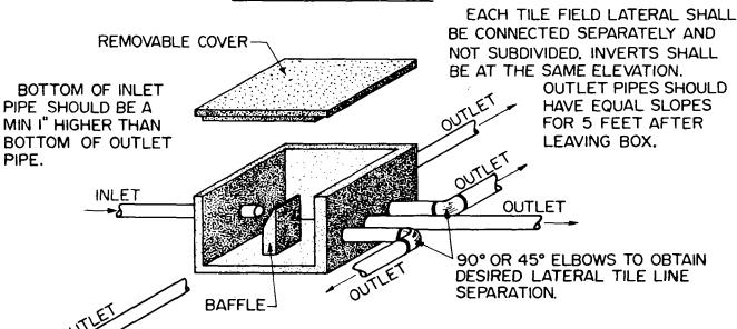
BAFFLE TO BE USED WHEN EFFLUENT IS DELIVERED BY PUMP OR SIPHON, OR THE SLOPE OF THE INLET LINE IS SUCH THAT UNEVEN DISTRIBUTION COULD OCCUR. TOP OF THE BAFFLE AT LEAST LEVEL WITH THE CROWN OF THE INLET PIPE.
