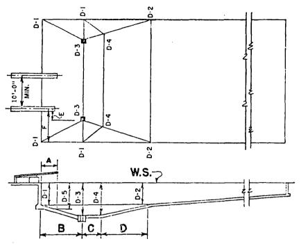
D-1 Shall be at End Wall of Diving Area or Not More Than 12" From This Wall.
