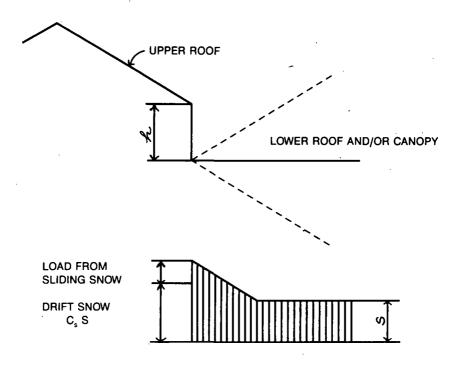
DESIGN LOWER ROOF OR CANOPY FOR LOADS ACCORDING TO FIGURE II + 50% OF DESIGN LOAD FROM UPPER. THE DISTRIBUTION SHOULD BE MADE DEPENDING ON THE RELATIVE SIZES, SLOPES AND POSITIONS OF THE TWO ROOFS.
