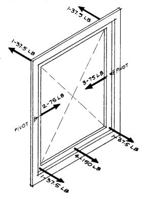
As shown, pivots are represented as triangles and sash pivots out from the bottom and in at the top.  $\label{eq:continuous}$
